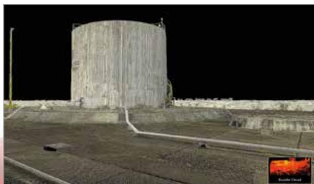
3D laser scanning, the time involved in tank inspections drops from weeks to hours – or even minutes. For example, the Leica RTC360, the fastest laser scanner available, completes a full scan in as little as 26 seconds.
